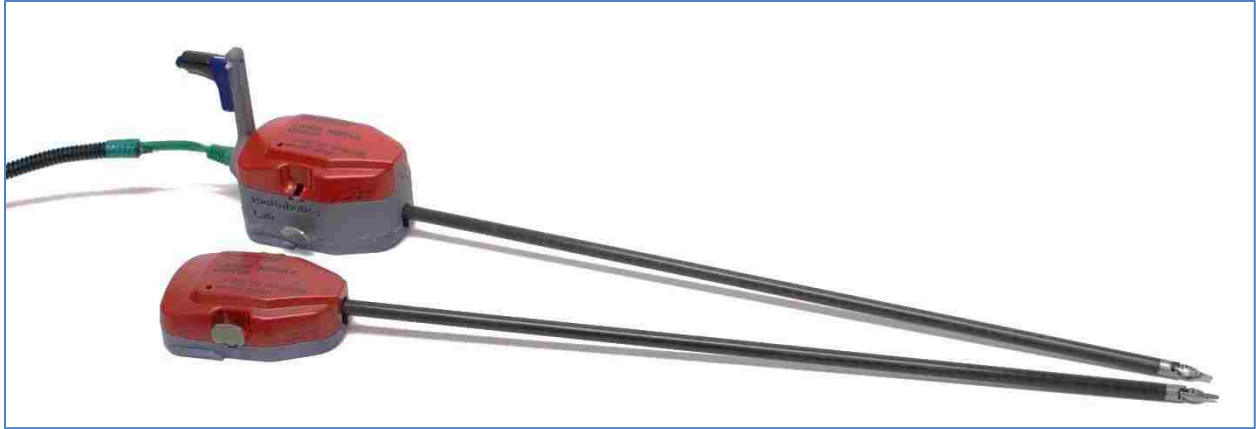
Figure 6 - SurgTrak modified large needle driver for the da Vinci Si.
