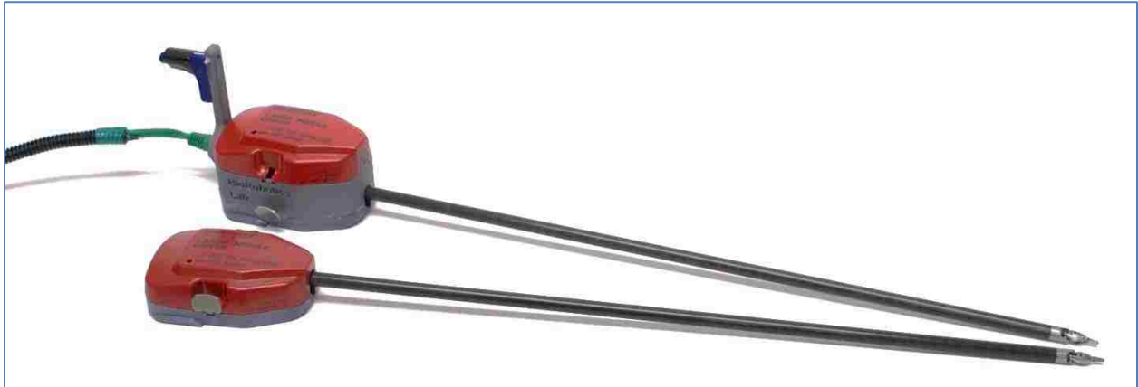
Figure 13 - Retrofitted da Vinci training instrument with sensor housing on back end.
